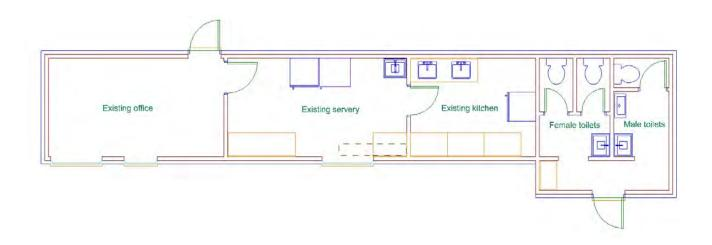
Our new proposed lay out would move the existing office to the new office built under the new start ramp allowing for a greater toilet area. Kitchen and servery area would be relocated with several upgrades to comply with current health standards.
