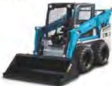
Skid Steer Loader – Toyota Huski 5SDK11 (900kg operating load capacity)
