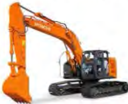
Excavator – Hitachi ZX225US-5 (122 kW)
