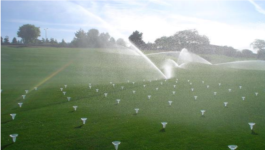
Catch cup test method
