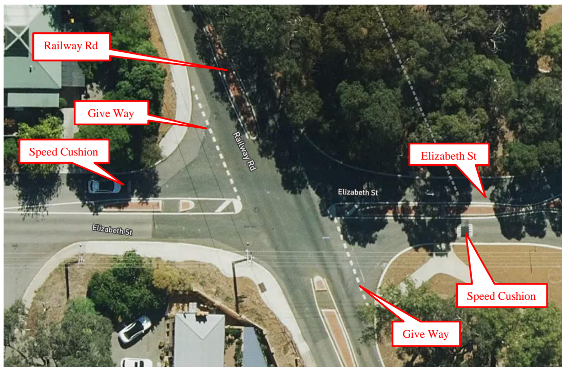
Figure 3.1: Current Intersection of Elizabeth St with Railway Rd is under Give Way Control
