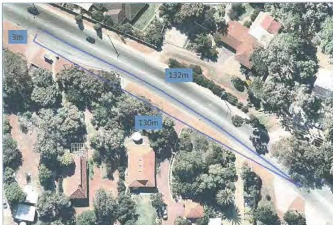
Figure 3.1: Access Driveway Visibility
